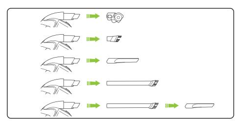
An active nozzle is built into your Multi. The dusting brush, crevice tool, extension tube and power brush all attach to the active nozzle.
