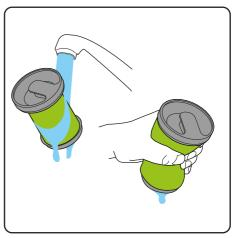
Wash the filter under a tap, squeeze it out then let it **dry completely** before using it. Recommended water temperature 40°C. Do not use any detergent or soaps. (You can buy more at **www.gtech.co.uk**) **Never put the bin back without the filter inside. You could damage the motor.**
